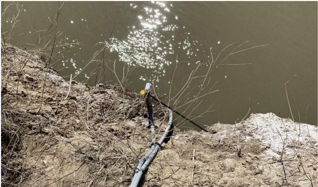
Figure 3.—Hydrophone mounted to rebar driven in to the riverbank; this is the “upper hydrophone”, the “lower hydrophone” is submerged; photograph taken by Rebecca Braz, 2021.
