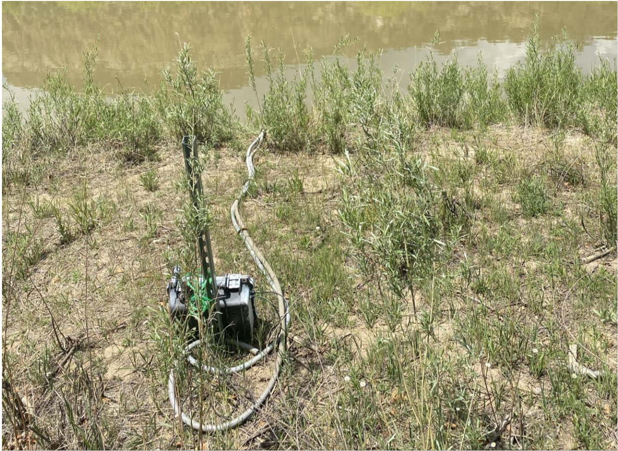
Figure 4.—A water-resistant case housed the data collector, pre-amplifier, and batteries at each site; the case was secured to a U-channel driven into the floodplain about 10 feet from the river's edge; photograph taken by Rebecca Braz, 2021.
